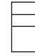
B pedestal (Full-length) - 2 box drawers - 1 file drawer - 1 pencil tray - drawer 1 is separated from drawers 2 and 3 by a solid horizontal piece - drawers lock together with one lateral lock
